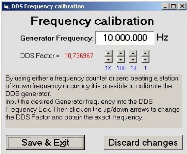
Adjust the DDS Factor with the UP/DOWN arrows to obtain the exact Generator Frequency in real time at the DUT connector. Save & Exit and continue with calibrating the Reflection/Transmission
