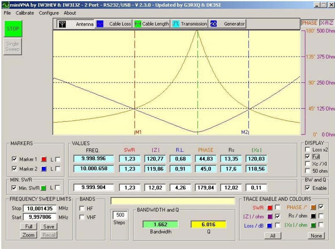
Connect the XTAL to the DUT connector and find at what frequency it has the lowest impedance. You may need to Zoom the frequency range a couple of times. The Q and Bandwidth can be found where the Phase is 45°
