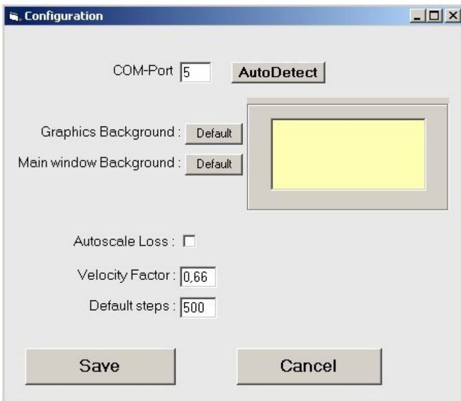
Use Auto Detect to identify and save the virtual Com-Port for the USB connection. If you want different Graphic or Background colours, click on the appropriate part of the frame and make your colour selection.
