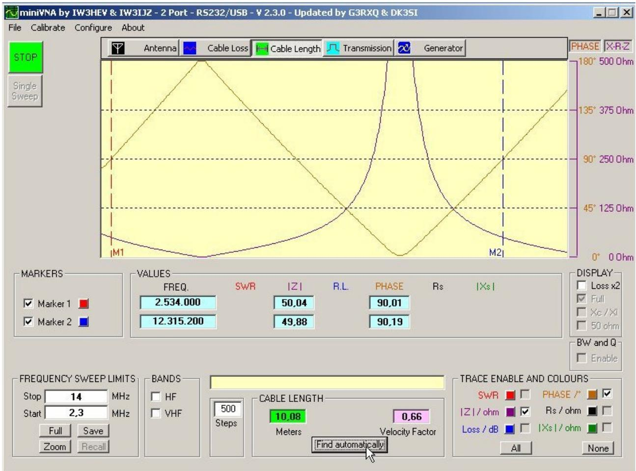
Connect the unknown cable to the DUT connector, then click the “Find Automatically” button. It will take some seconds until you see the correct length. The cable length is calculated from adjacent Phases at +90° and dependant from production tolerances of the Velocity Factor. It is still possible to set the needed 2 Markers and measure manually. Do not try to measure with a Single Sweep.
