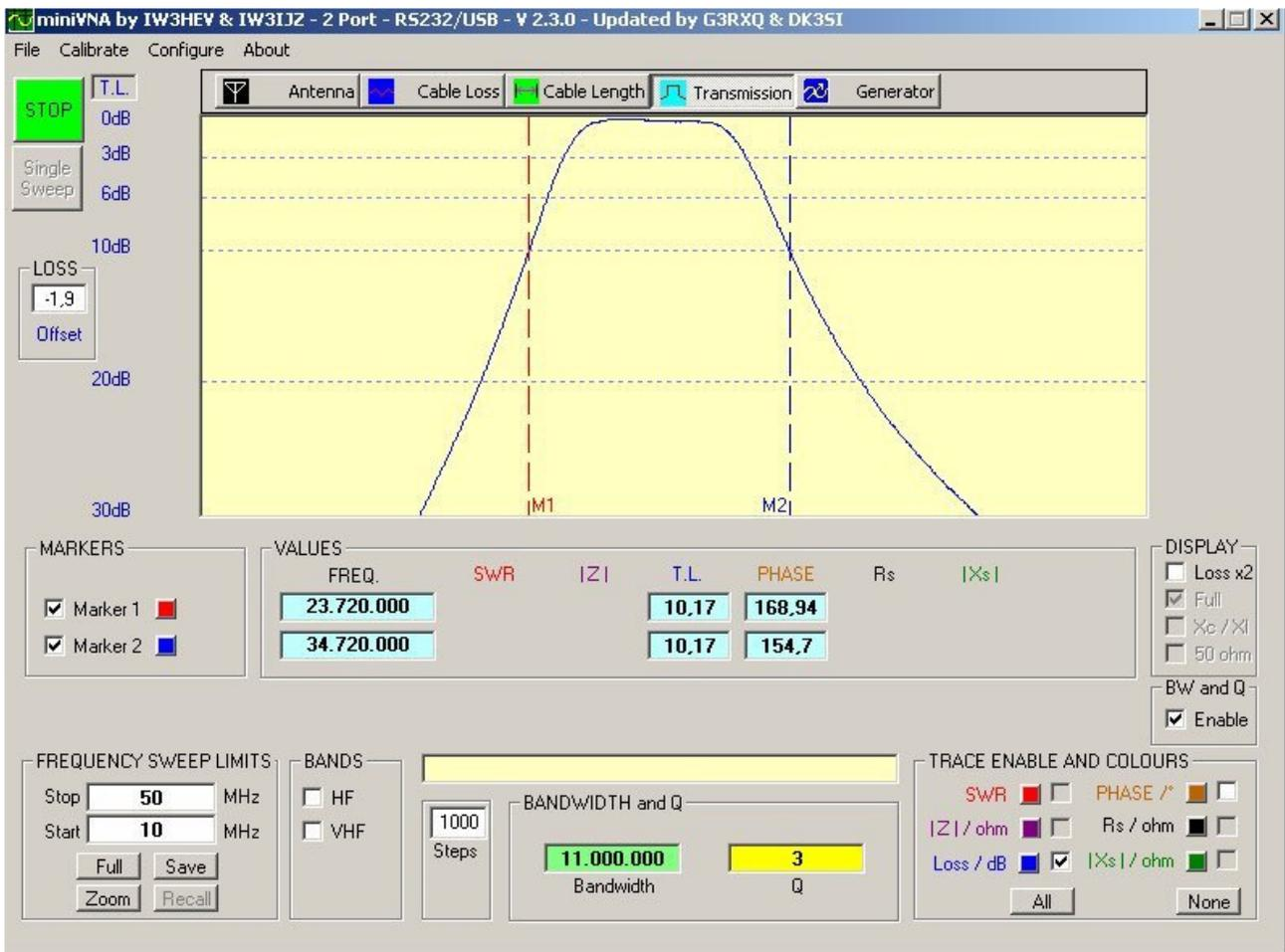
Connect the filter between DUT and DET. If it has an Insertion Loss you can compensate it in the Loss Offset box. To view the 3/6/10dB Bandwidth, just set both markers and enable the BW&Q.
