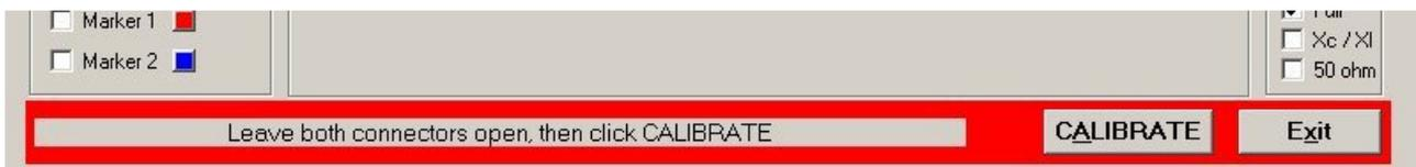
The Calibration procedure for Open condition takes some seconds. Crosscheck the SWR or Return Loss afterwards with a good 50 Ohm reference on the DUT connector.
