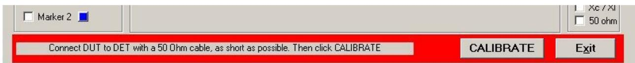
As above, wait some seconds until you see the Save message. The Return Loss should be near to Zero dB in Transmission Mode. Check that with the short cable in Transmission Mode afterwards.
